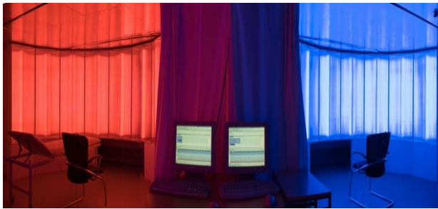
Figure 1: Configuration of light cabins: The testing room with red and blue light scenarios is shown.
