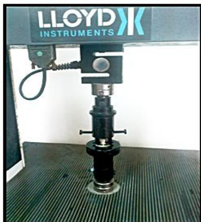
Fig. 6: Close-up view to specially designed attachment in universal testing machine
