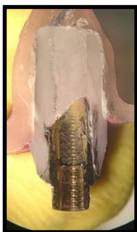
Fig. 7: All-ceramic crown cemented with Rely-x luting cement. This specimen was given a score of 1. (The die penetrated along the gingival wall)
